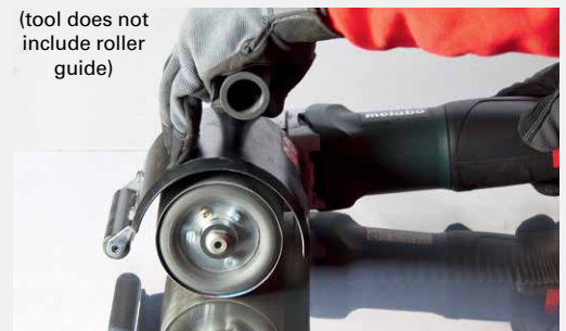
Preparation for mirror polishing: Metabo Burnishers with expansion roller, and Pyramid sanding belts from A160 (120 grit) to A6 (2000 grit).
