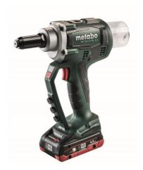
The 18V Brushless Rivet Gun (NP 18 LTX BL 5.0) is perfect for securing steel/stainless steel or aluminum in place. It can rivet up to ½" in aluminum and 3/16" in steel. With a compact 4.0 Ah LiHD (Lithium High Density) battery, it can secure 2,000 3/16" rivets on a single charge and has a pulling force of 2,250 lbs.
