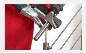
The Pipe and Tube sanders for a uniform even finish on hand rails using Pyramid sanding belts from A160 (120 grit) to A6 (2000 grit).
