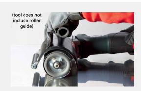
Preparation for mirror polishing: Metabo Burnishers with expansion roller, and Pyramid sanding belts from A160 (120 grit) to A6 (2000 grit).
