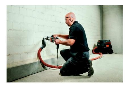
Metabo offers an extensive range of system accessories for all machines in the new drill range. For the effective extraction of mineral dusts, users combine for example the vacuum cleaner adapters DDE 14 or DDE 72 with an M-class all-purpose vacuum cleaner. Photo: Metabo
