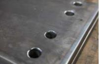
Before (left), after (right): the main application at Unger is the cutting of a radius for bores in steel components in preparation for a high-quality corrosion protection coating. Photo: Metabo
