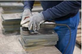
The compact bevelling machines are comfortable to use and can be adjusted easily without using tools. The edges of six bores in a steel structure sheet are cut within 60 seconds. Photo: Metabo
