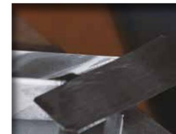
Use the stainless steel tape to mask off the fresh burnished area. Make sure it is fixed securely. Thus protecting the mitre joint from the next step.
