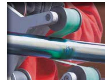
Use either the corded or cordless RB machines with the ceramic grain P 80 grit sanding paper to remove the weld in one step. The ceramic grain paper offers high material removal rates together with extremely long life. Select high speed setting 6\* and remove a TIG weld seam in seconds.
