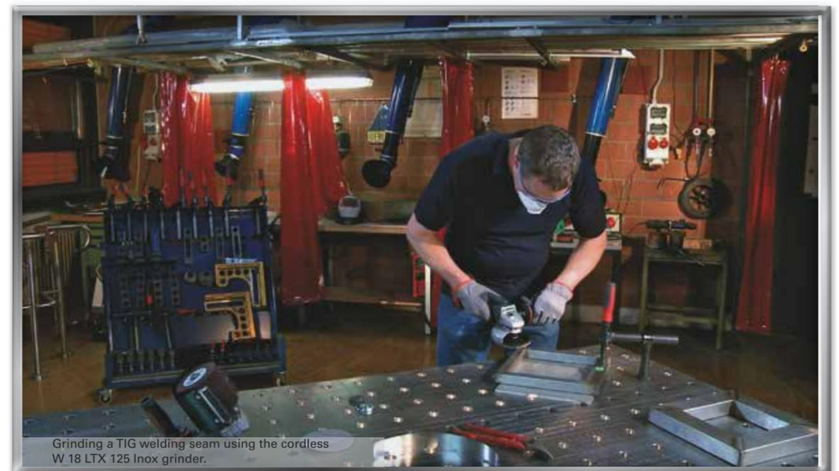
Grinding a TIG welding seam using the cordless W 18 LTX 125 Inox grinder.
