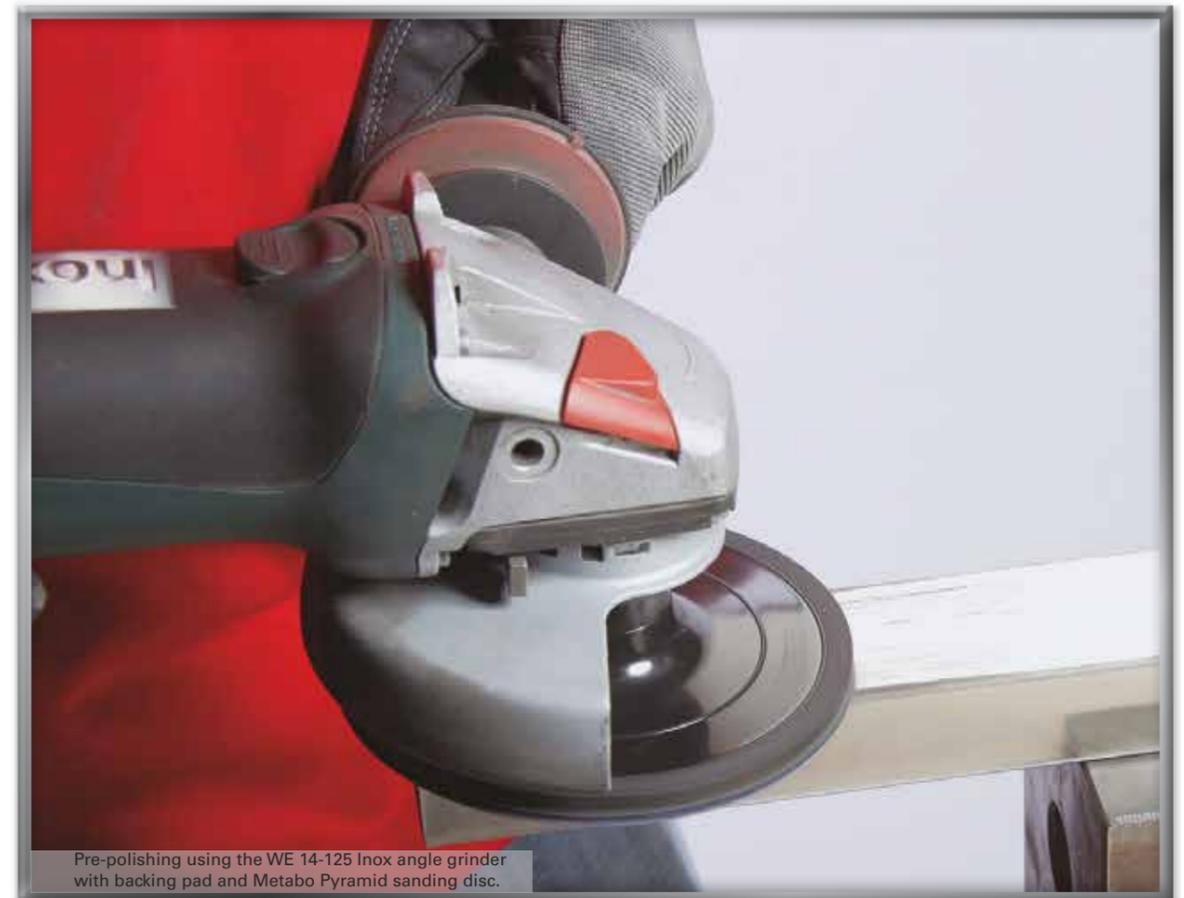
Pre-polishing using the WE 14-125 Inox angle grinder with backing pad and Metabo Pyramid sanding disc.
