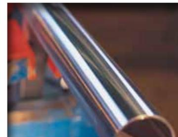
This shows a surface which has been pre-ground to Pyramid belt grade A6, P 2000. The surface is now silky smooth with a high sheen finish. With this finish we are now at the perfect stage to start polishing.
