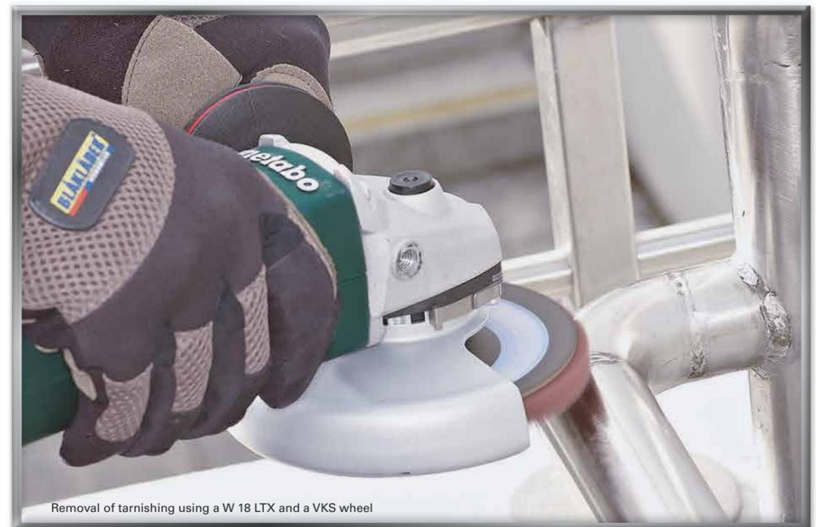
Removal of tarnishing using a W 18 LTX and a VKS wheel
