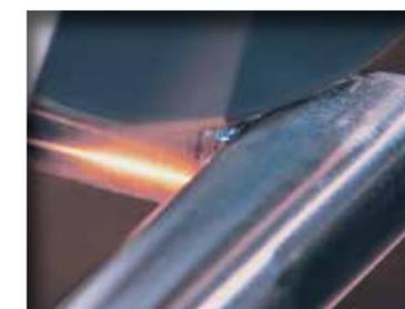
The KNS fillet weld grinder is the machine of choice for this task thanks to its ultra slim profile. Select speed setting 5\* and remove the fillet weld seam easily, even right into the corner without damaging neighbouring surfaces.
