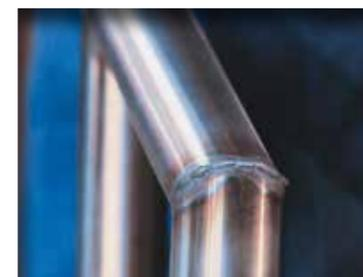
TIG welding seam on a handrail corner.
