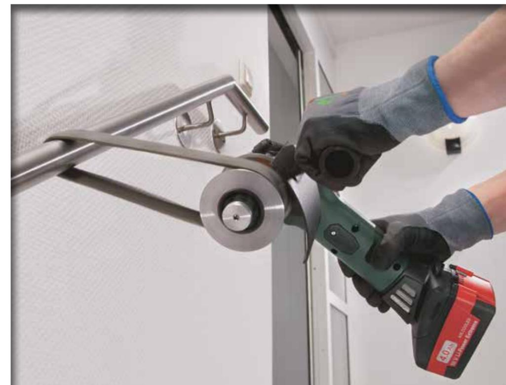
For closed off rail sections close to a wall the Metabo belt drum and "buttonhole" belt accessory option will prove particularly useful, especially if the rail is closed off with wall brackets on either side of your working area. With the buttonhole belts you can then loop & close the belt behind the rail. With this method you will achieve a perfect uniform result 360o around the handrail. Going mobile? Go cordless with the S 18 LTX 115.
