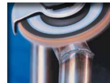
Using the KLS wheel you can remove the weld and achieve a high quality surface finish in just one step. Due to the tough yet flexible nature of the KLS wheel you can work with the form of the pipe profile. Select speed setting 3\* and work in the direction of the pipe.
